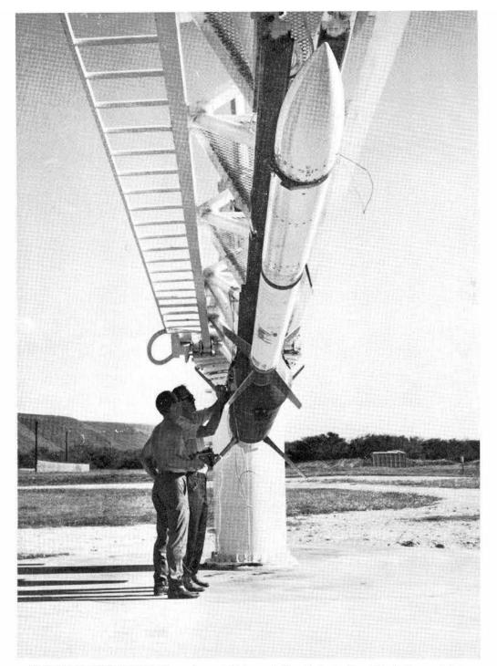
CHECKING FIRING CIRCUITS are Roger Gelder and Jim Malloch. The Nike-Cajun rocket is assembled with the payload on the launcher and almost ready for firing. The launcher can be raised to any angle and aimed for the proper rocket trajectory.
